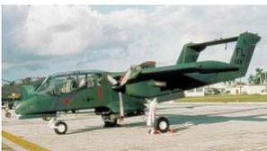
Later, the OV-10 Bronco military aircraft was brought in as a FAC aircraft. It was designed by the military for aerial recon and target missions. It flew 2 to 3 times faster than the O-2, and carried rockets and a machine gun.
