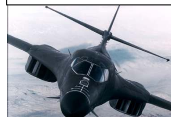
B-1 with wings swept back for transonic speed
