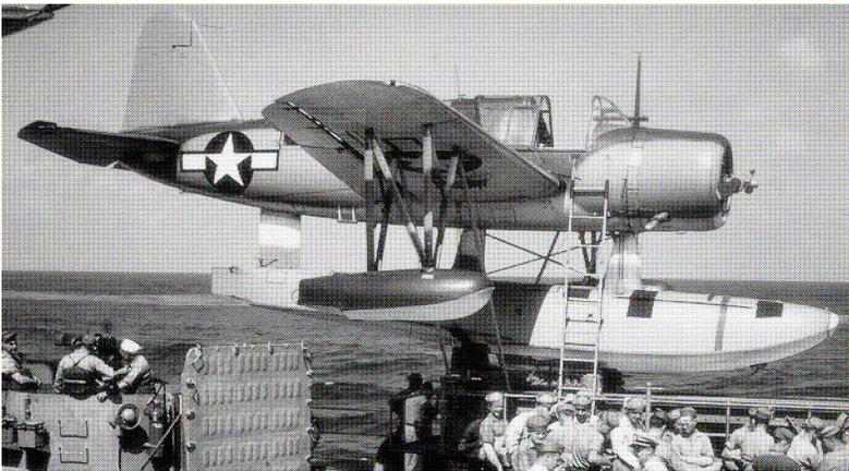
At the time of Pearl Harbor attack, all Navy battleships were equipped with the floatplanes for spotting of naval gunfire and general observation. They were gradually replaced by radar. **Lt. (jg) Huston** was assigned to the Battleship USS Colorado. The USS Colorado had two Kingfisher planes and a launching rail. During the November 1943 battle for Tarawa Atoll, he was flying spotting duty and observed the Marines as they tried to make an amphibious landing on the beach. He could see
